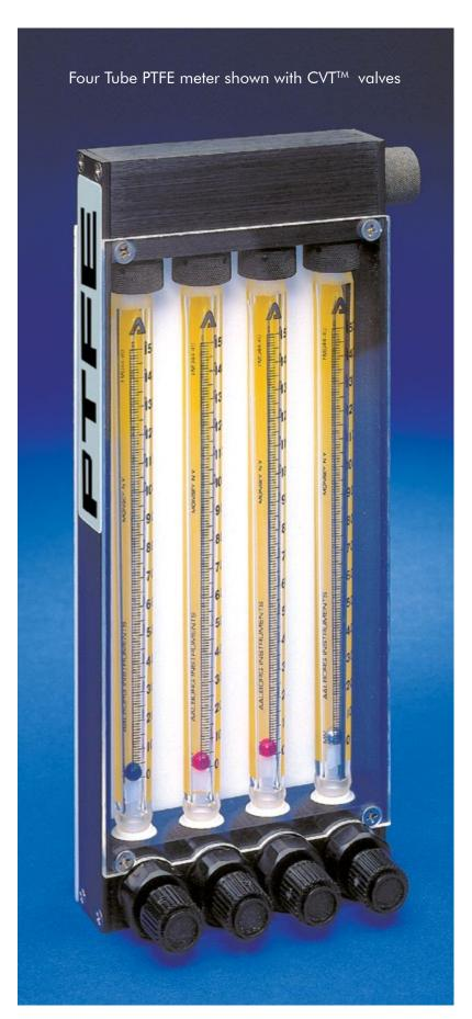
Model Tx Multiple Tube PTFE-Glass Flow meters combine the convenience of multiple tube meters with the unique design features of single tube PTFE-Glass flow meters. These meters are available with the same interchangeable 65mm or 150mm glass flow tubes used in single tube designs and they are available with or without built-in PTFE needle valves.
